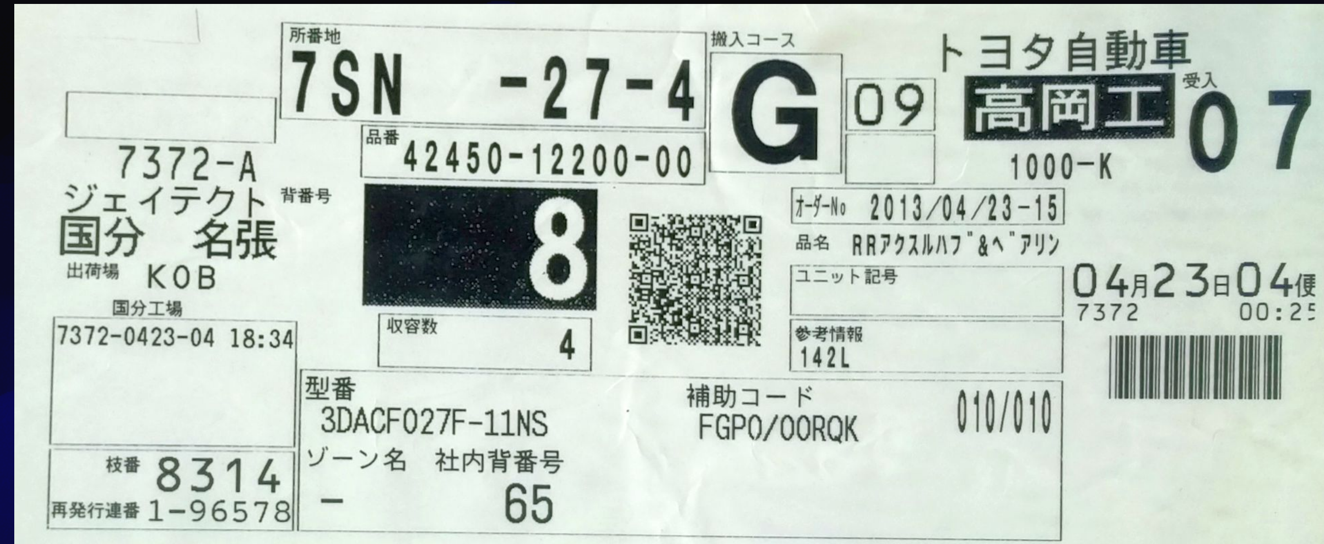
Image: Example of a Toyota Kanban Card for delivery of axle hub and bearings from JTEKT to the Takaoka plant of Toyota.
